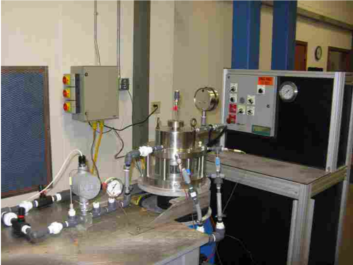
Figure 7 SVTR Test Head and Low Flow Hydraulic Pump
