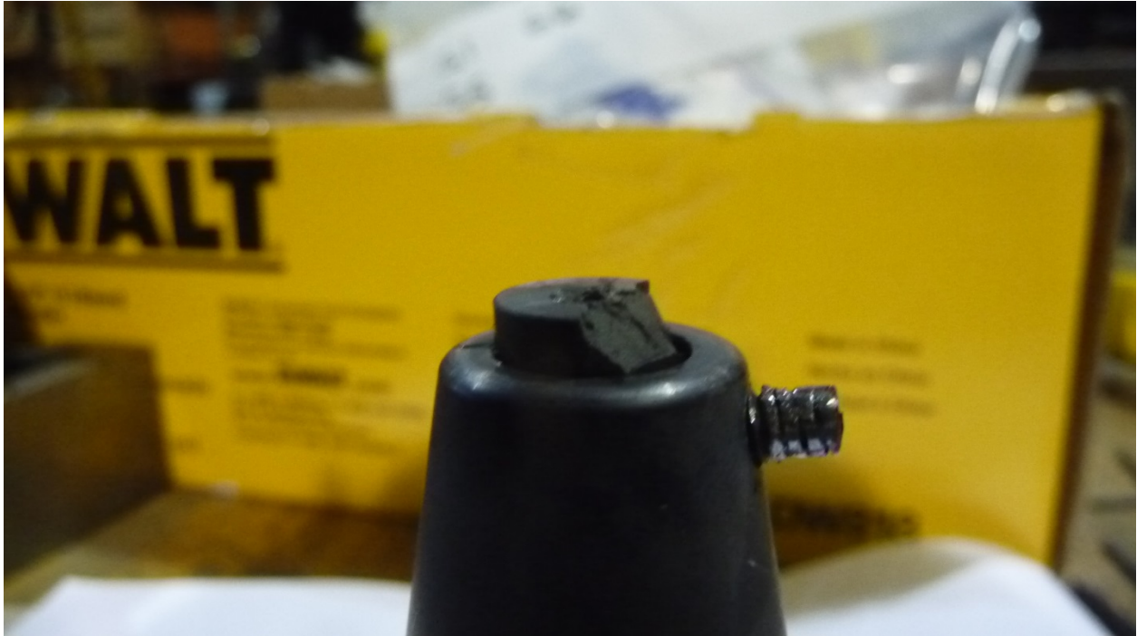
Figure 31: G1-1 After Fracture Failure During Weld Number 20
