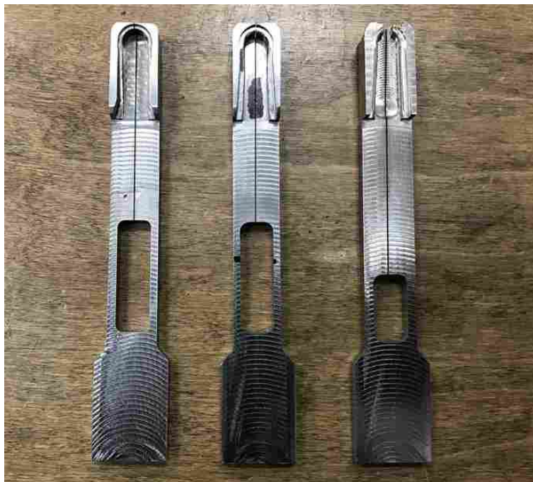
Figure 30 Feed Tray Iterations: Gen 1 (Left), Gen 2 (Center), and Gen 3 (Right)
