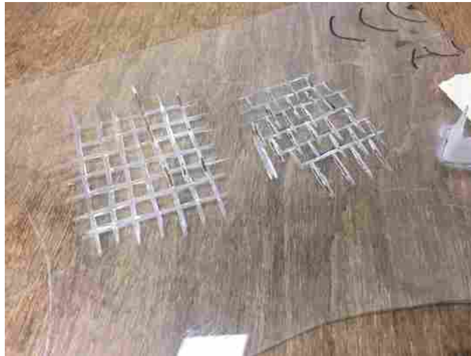
Textured Surface Used for Bit Orientation Testing
