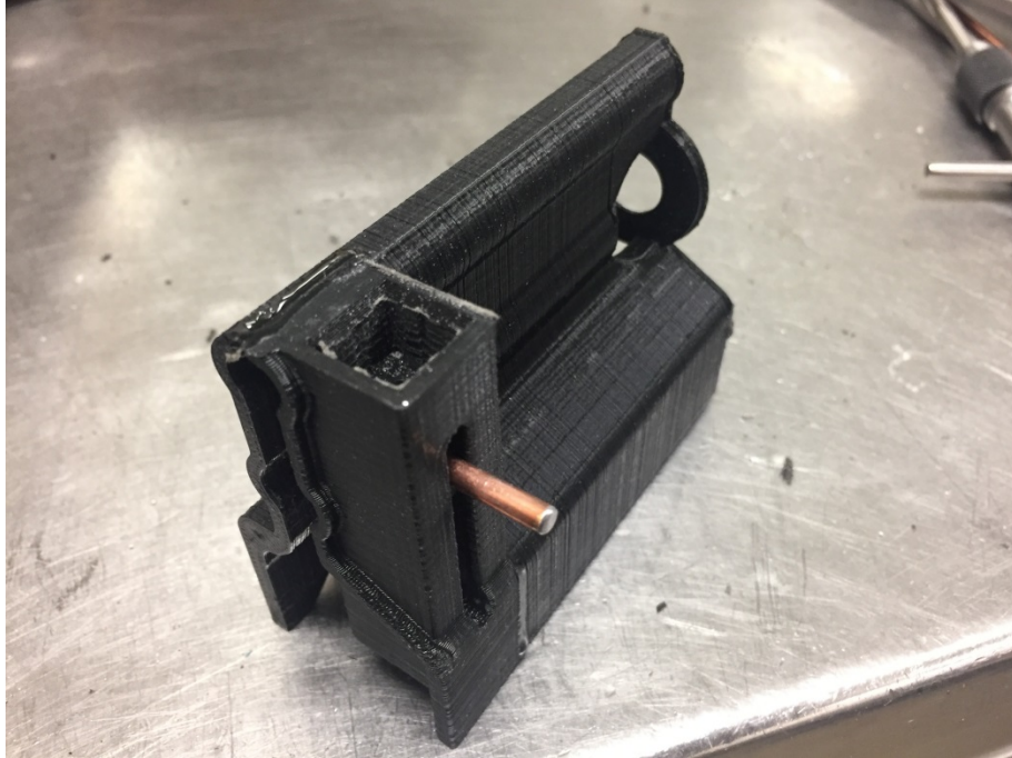
An Early Prototype Frame that Housed the Magazine and Bits
