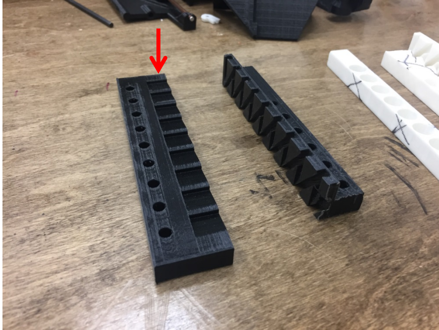
Early Straight Magazine Prototype, Ratchet Teeth Indicated by Red Arrow
