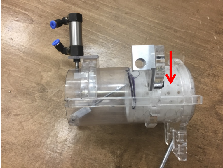
Early Feed System Prototype with Helical Magazine (Red Arrow)
