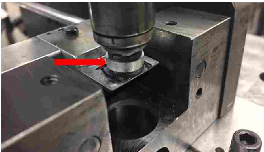
Magnetic Loading Lever in the Up Position, Magnetic Cup Indicated by Red Arrow
