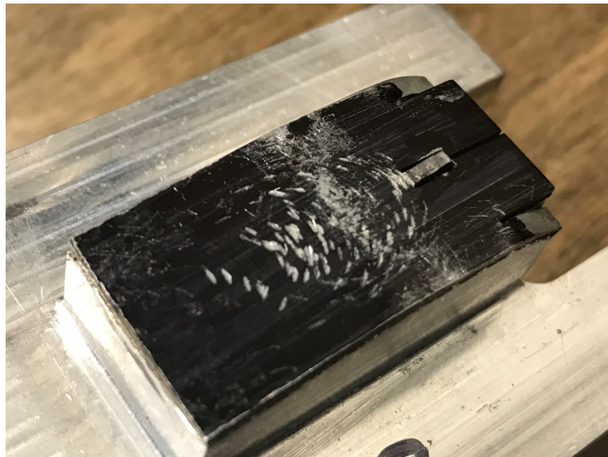
Figure 37 Pin Skid Plate Wear Pattern, Marked with Dye
