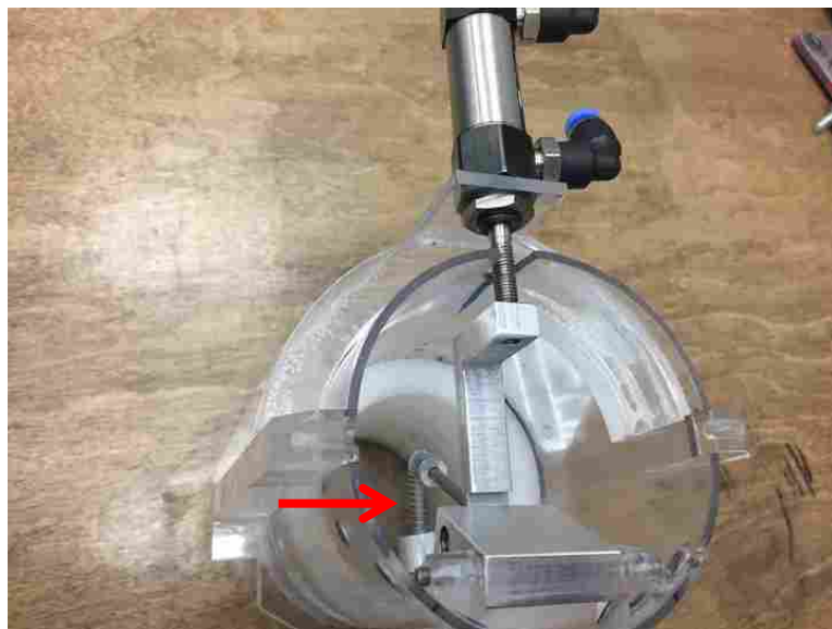
Inside the Early Prototype Feed System, Bit Armature (Red)
