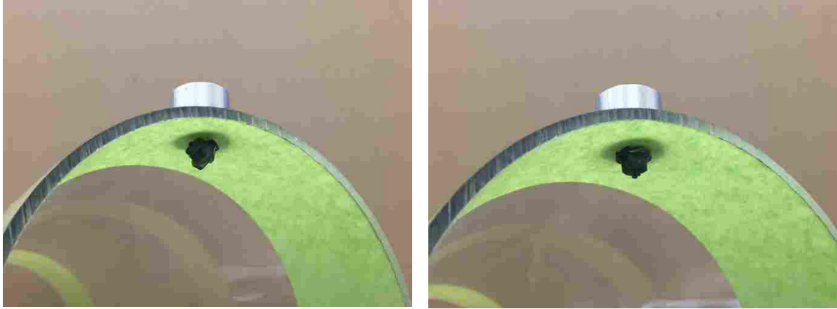
Magnetic Drag Experiment, Disoriented Bit left, Oriented Bit Right
