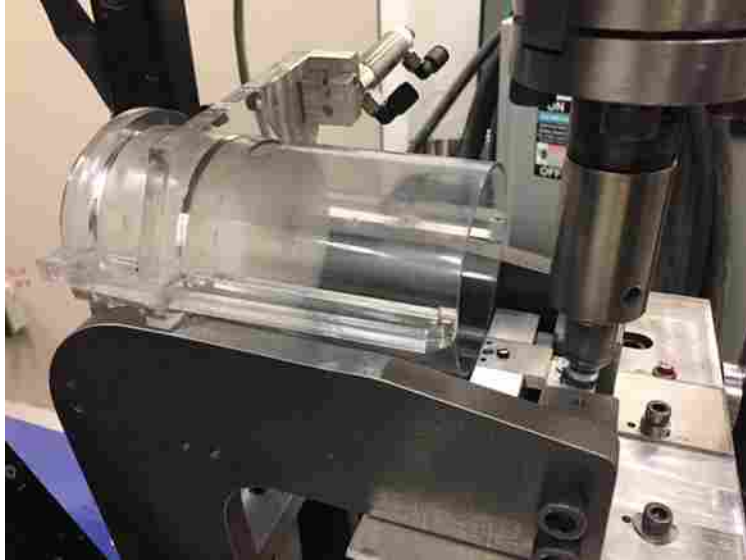
The Feed System in its Installed Position in the FBJ Welder
