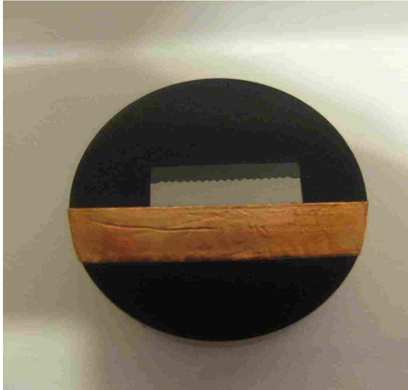
Figure 4-12: Sample prepared for SEM analysis.
