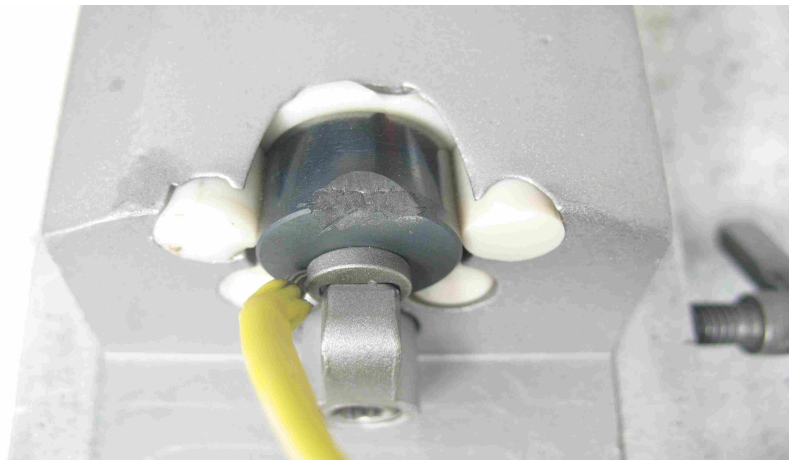
Figure 3-10: PDC insert in the testing fixture after heavy wear test.
