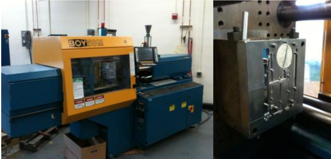
Figure 3: BOY 50M Injection Mold Machine (left) & Mold for Type 1 Tensile and Falling Dart Impact Samples (right)
