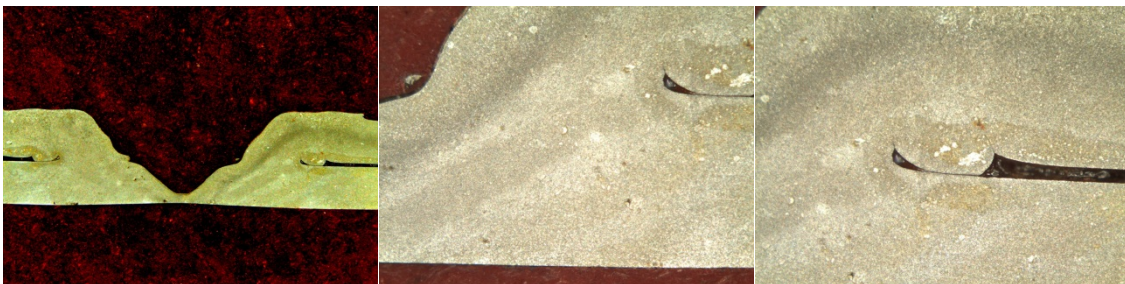
Figure 3.12: Three Examples of Pictures Taken with a Microscope. From Left to Right the Pictures Show the Geometry, the Bond Area, the Welding Hook, and All of them Show the Microstructure
