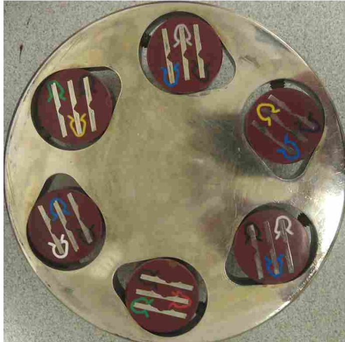
Figure 3.10: Polishing Wheel with Samples Mounted
