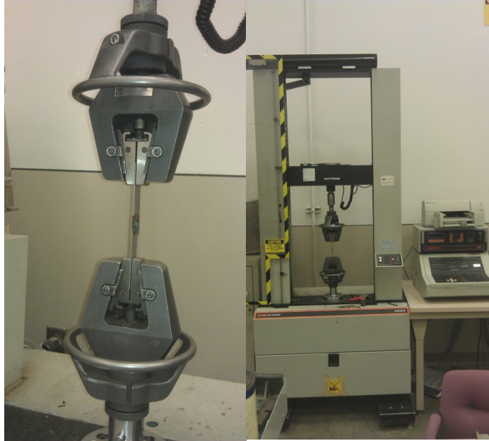
Figures 3.3 a) & 3.3 b): Close Up of Lap Shear Tensile Test and Instron Tensile Tester
