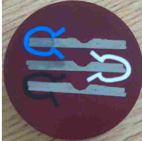
Figure 3.9: Bakelite Sample with Three Weld Profiles
