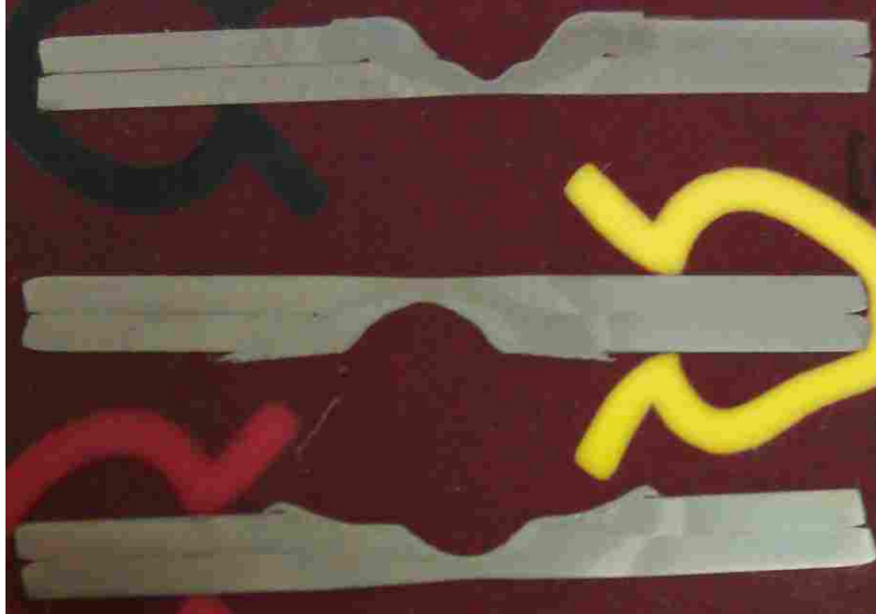
Figure 3.11: Polished Cross Sections with Nital Etching
