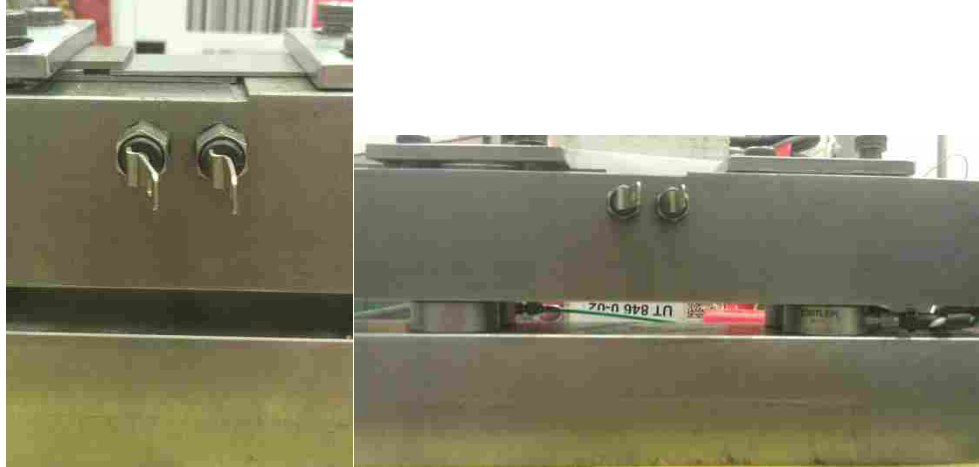
Figures 3.4 a) & 3.4 b): Lap Configuration and a View of the Load Cells
