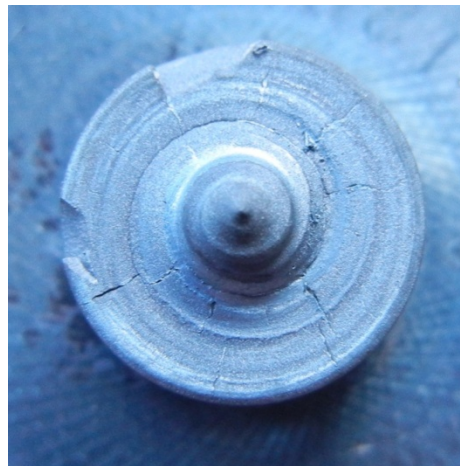
Figure 4-2: Chipped Shoulder and Radial Cracks of PCBN MS80 SN2235
