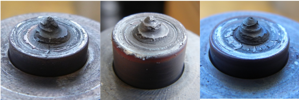
Figure 4-18: MS 80 J1, SN2236, J2 Welding Tools at Weld 700
