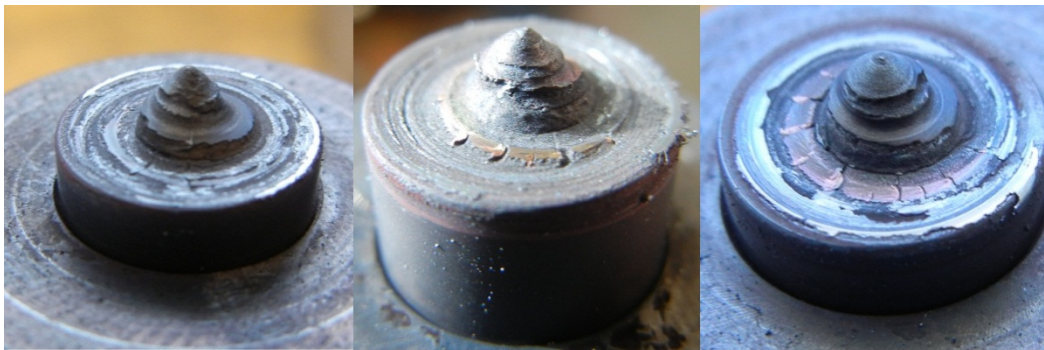
Figure 4-16: MS 80 J1, SN2236, J2 Welding Tools at Weld 500
