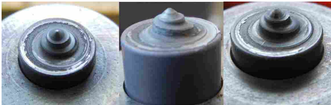
Figure 4-12: MS 80 J1, SN2236, J2 Welding Tools at Weld 100
