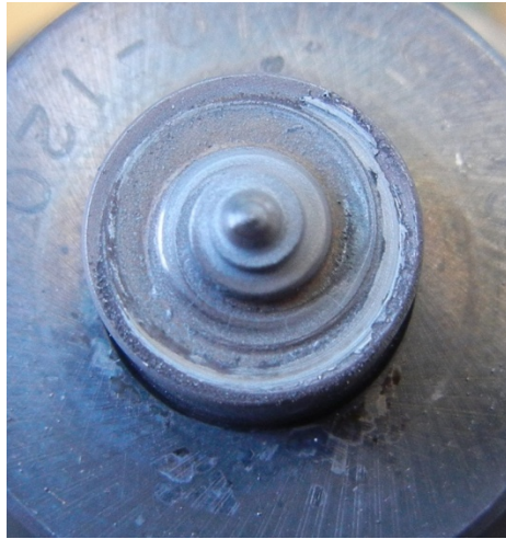
Figure 4-3: Material Build-up on MS80 PCBN Tool at 45 Welds
