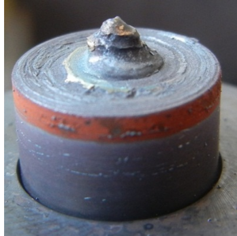
Figure 4-1: Red Oxide Layer on MS80 SN 2236 After 800 Welds
