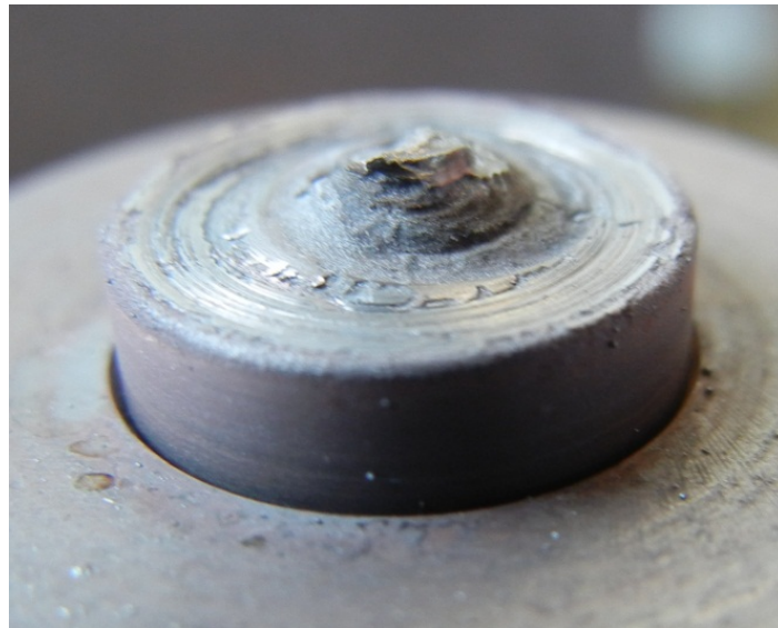
Figure 5-1: Failed MS80 J1 PCBN Tool After 976 Welds
