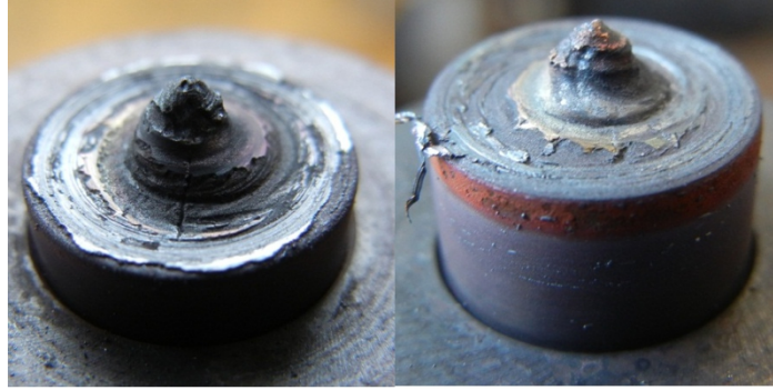
Figure 4-20: MS 80 J1, SN2236 Welding Tools at Weld 900
