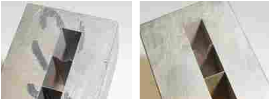
Figure 4.2 - Test Specimens Demonstrating a Notch Defect in the Thin-walled Section
