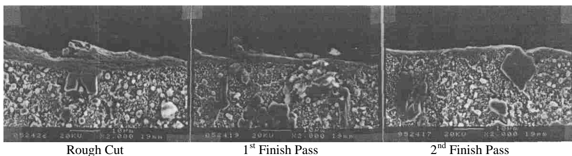
Figure 2.10 - Magnified Pictures of the Recast Layer 48
