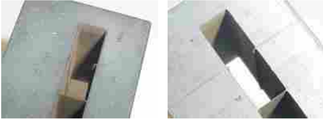
Figure 4.1 - Test Specimens Demonstrating a Defect where a Thin-walled Section is Depleted
