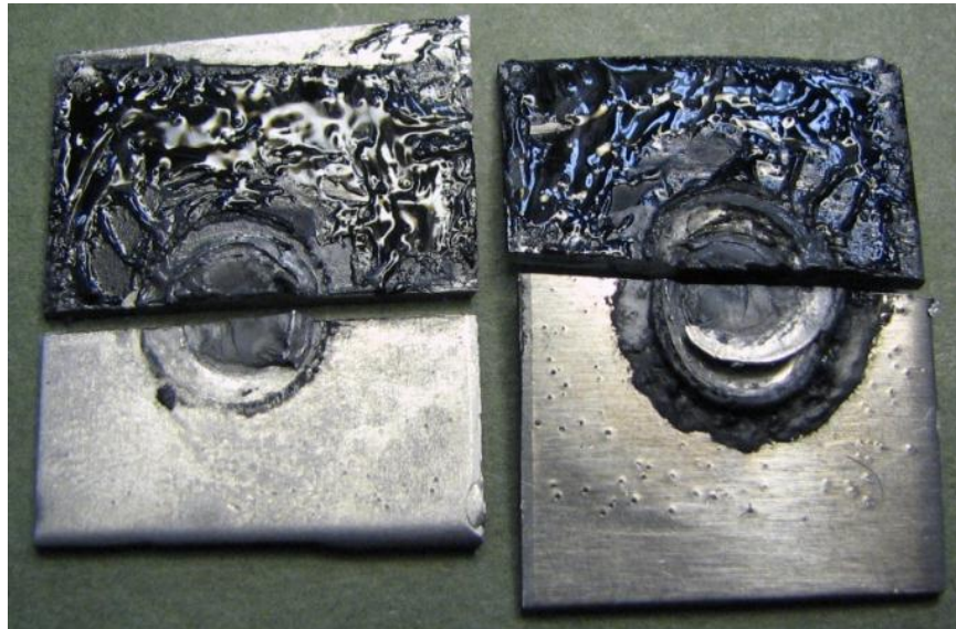
Figure 14: Weldbonded Shear Samples Showing the Cured Adhesive
