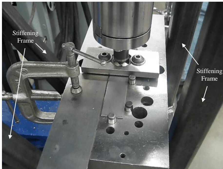
Figure 13: Friction Bit Joining Machine with Stiffening Frame
