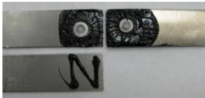
Figure 8: Adhesive Application for Weldbonded Specimens
