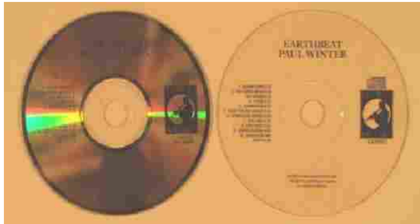
Figure 2-12: Oxidation of CDs after 500 Hours of Accelerated Aging (Shahani, Manns and Youket 2004)
