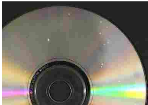
Figure 2-7: Corrosion of Reflective Layer (Shahani, Manns and Youket 2004)
