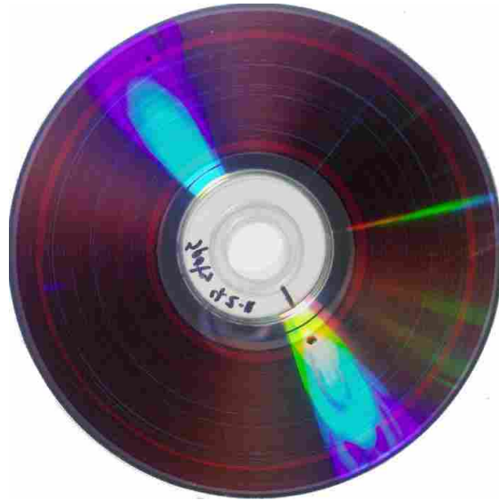
Figure 4-3: Two Mark Disc Image Overlaid on PIE Errors
