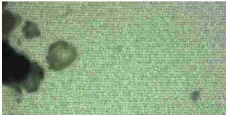
Figure 2-9: Close-Up View of Effects of Corrosion Damage on Data (Shahani, Manns and Youket 2004)
