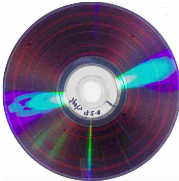
Figure 4-5: Four Mark Disc Image Overlaid on PIE Errors
