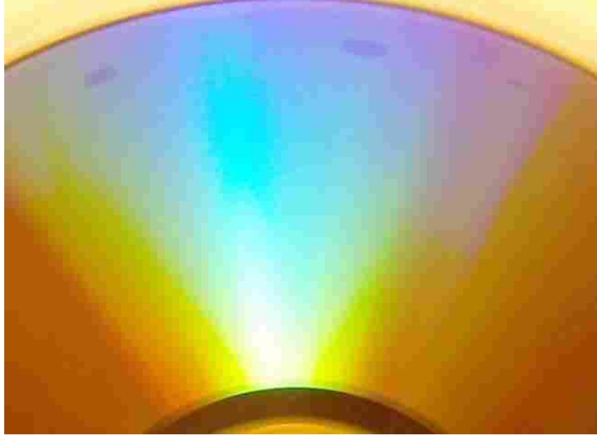
Figure 4-11: MI1 Black Spot Defects at 24 Hours
