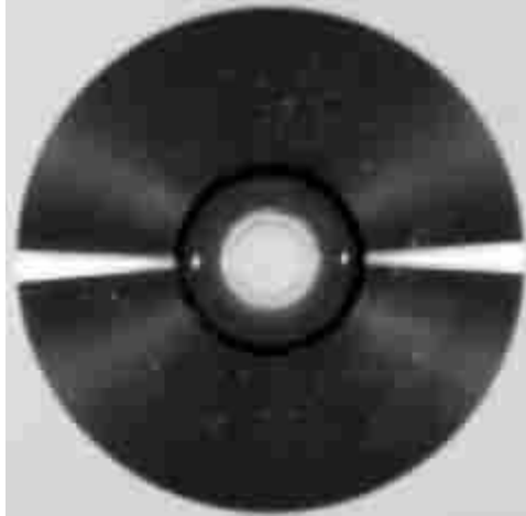
Figure 2-11: Example of Pinholes in Reflective Layer (Iraci 2005)
