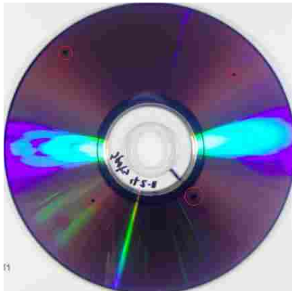
Figure 3-20: SectorDraw Validation Disc with Four Marks
