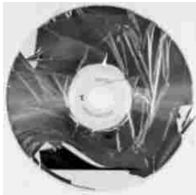
Figure 2-16: CD-R Delamination after 21 Days of Aging (Iraci 2005)
