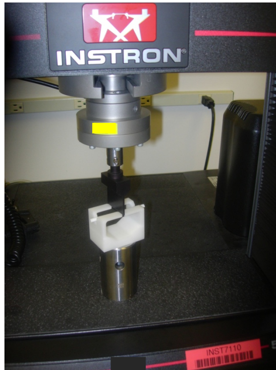
Figure 5 - Instron Machine with Tubing Segment Undergoing Stiffness Testing
