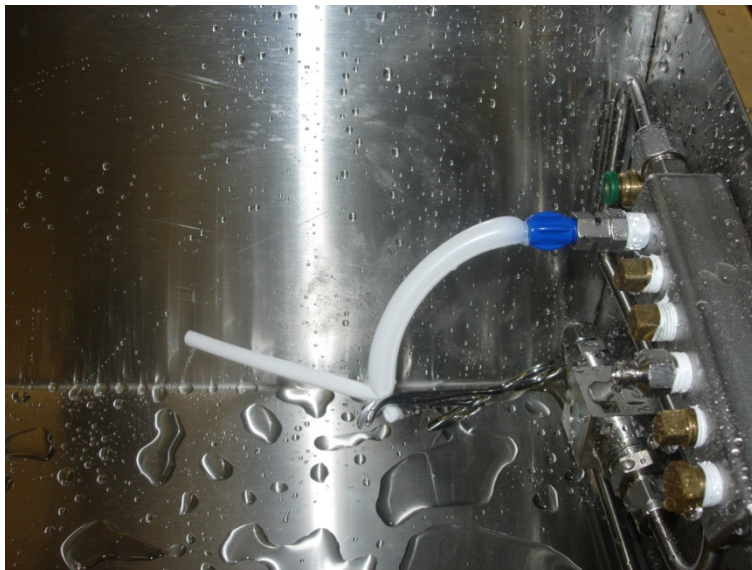
Figure 9 - Tubing Segment Undergoing Hydraulic Burst Resistance Testing
