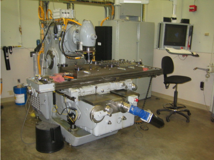
Figure 3-1 friction stir welding machine at Brigham Young University
