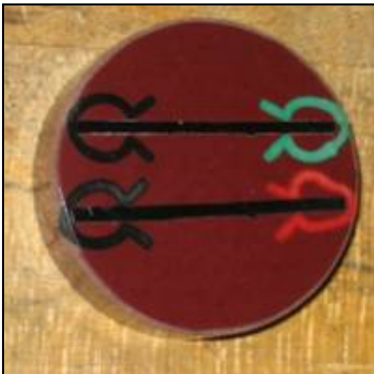
Figure 3-7 Two samples mounted in Bakelite.
