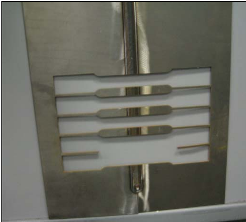
Figure 3-4 Welded sheet with tensile and hardness samples removed.
