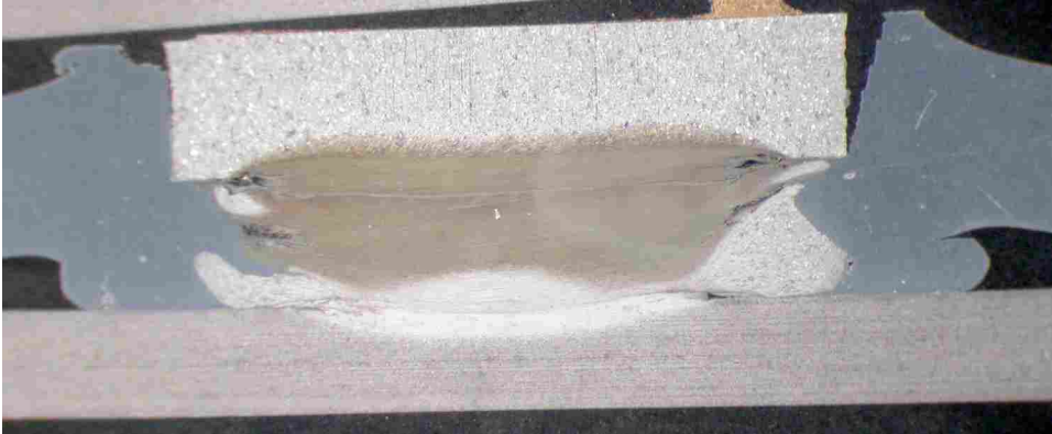
Figure 4.6 – Microscopy image of initial joint showing void at interface
