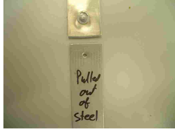
Figure 4.13 – Steel pullout failure
