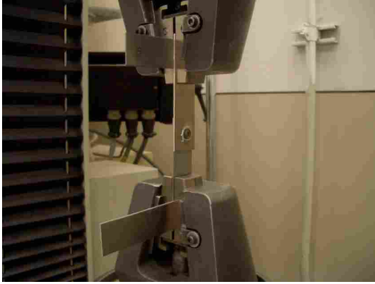
Figure 3.8 – Lap shear tensile test
