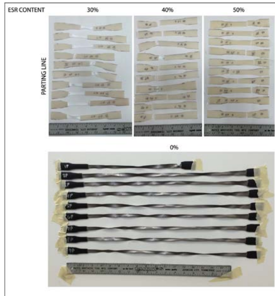
Figure 16: Parting Line Test Samples
