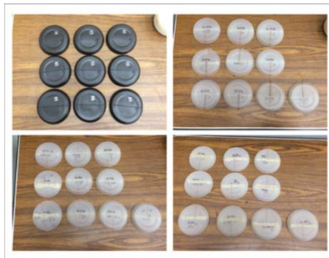
Figure 8: Bottle Samples (Upper left 0% ESR, Upper right 30% ESR, Lower left 40% ESR, Lower right 50% ESR)
