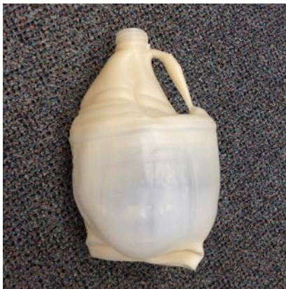
Figure 12: Sidewall Defect, Example 1
