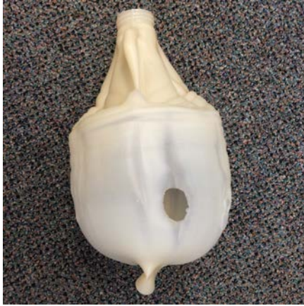
Figure 13: Sidewall Defect, Example 2
