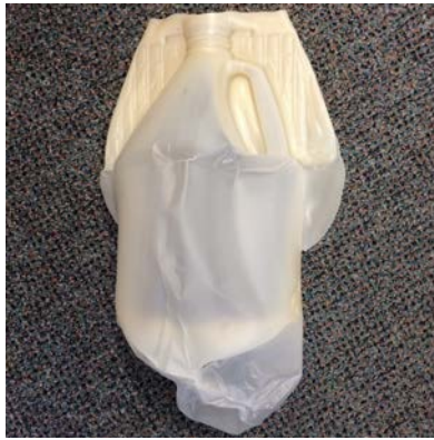
Figure 11: Example of Bottom Defect
