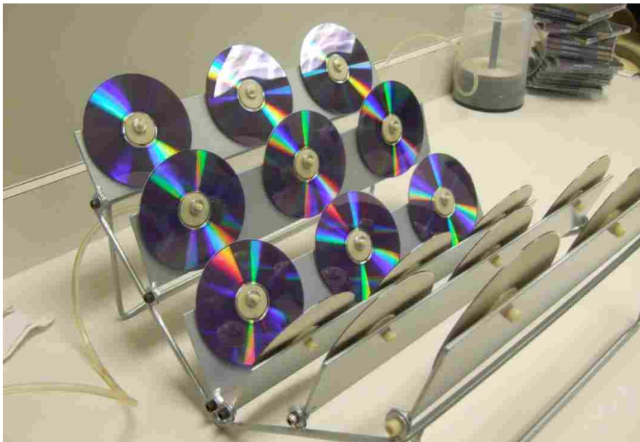
Figure 3.3 – DVD-Rs installed on the test rack. The angles were later adjusted to be completely vertical before placing the rack in the chamber.
