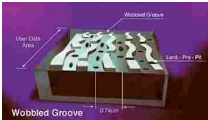
Figure 2.4 – A computer image of DVD-R track features. Source: Worthington 2005a, slide 6.
