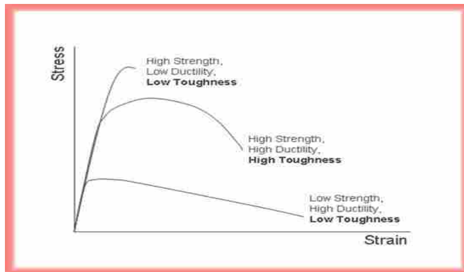
Figure 4-8 Stress-Strain Curve and Associated Mechanical Properties
