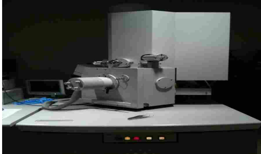
Figure 3-6 SEM-EDX Used for Chemical Testing
