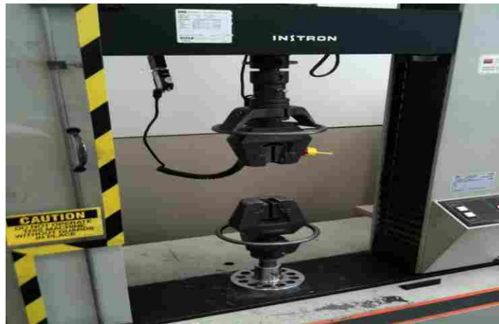
Figure 3-5 Instron Tension Machine Used for Mechanical Testing
