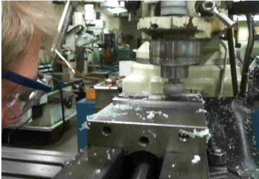
Figure 3-4 Mill Polishing Samples
