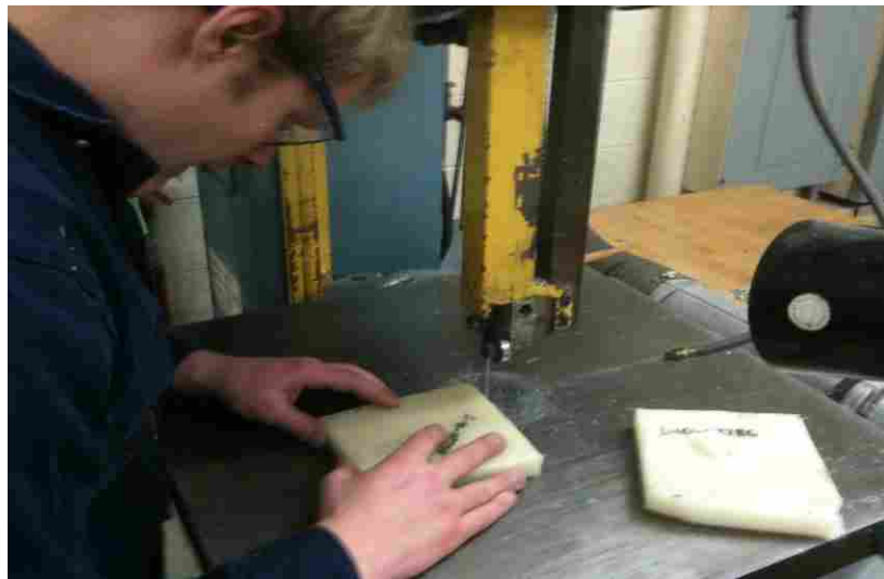
Figure 3-3 Bandsaw Cutting Samples
