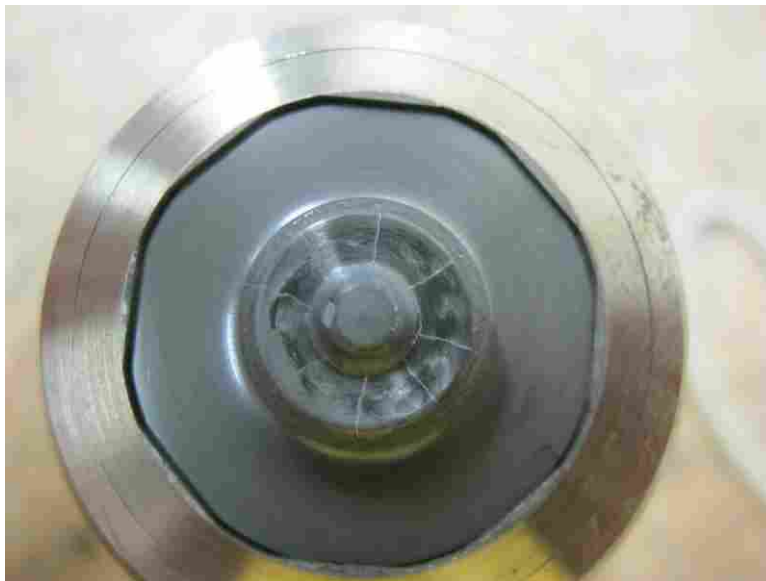
Figure 17: Cracking in PCBN Tool at 250 Welds
