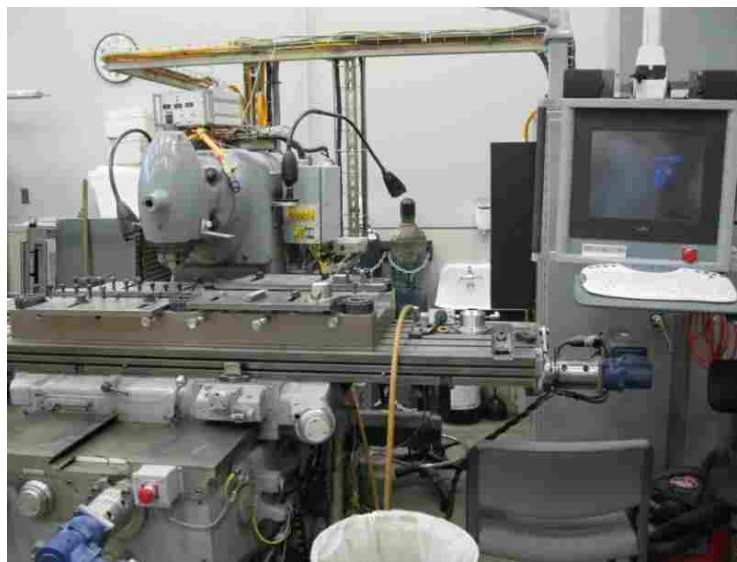
Figure 7: Kearney and Trecker CNC Mill
