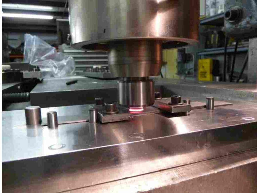
Figure 9: Friction Spot Welding of 4" x 1" Coupons for Lap Shear Testing
