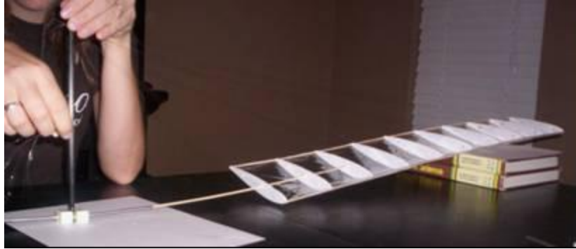
Figure 6-4 Re-rigging Rotors to add 10° of Anhedral Angle
