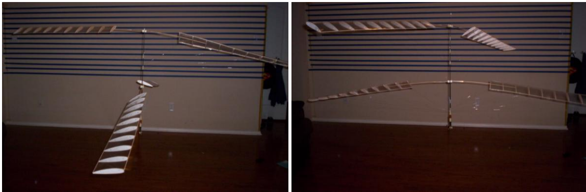
Figure 6-9 Coaxial Rotors in Motion, No Interference
