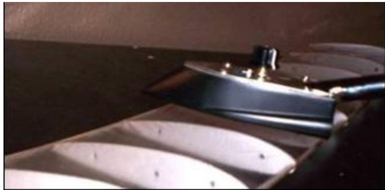
Figure 4-4 Hot Iron Application of Microfilm
