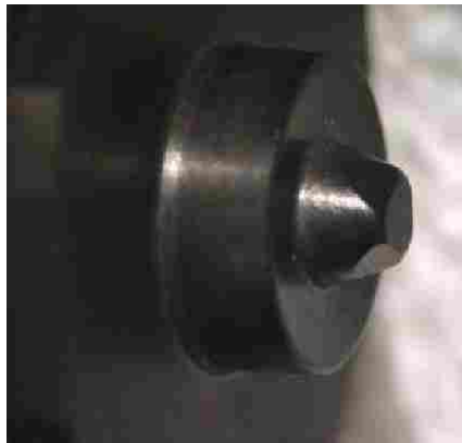
Figure 29: Example of a PCBN SFW tool. [25]
