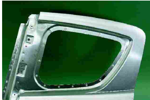
Figure 22: FSW in the rear door of the 2003 Mazda RX-8. [1]
