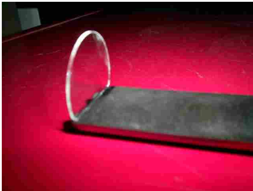
Figure 3-15 Sample holder with bare glass sample installed
