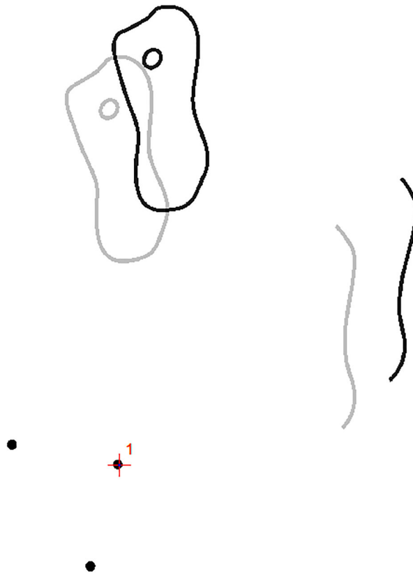
Figure 3. Illustration of the hypothetical examples in overlay format. Reference map A on top and map B underlying in grey. The three points in the bottom left corner are located on top of each other.
