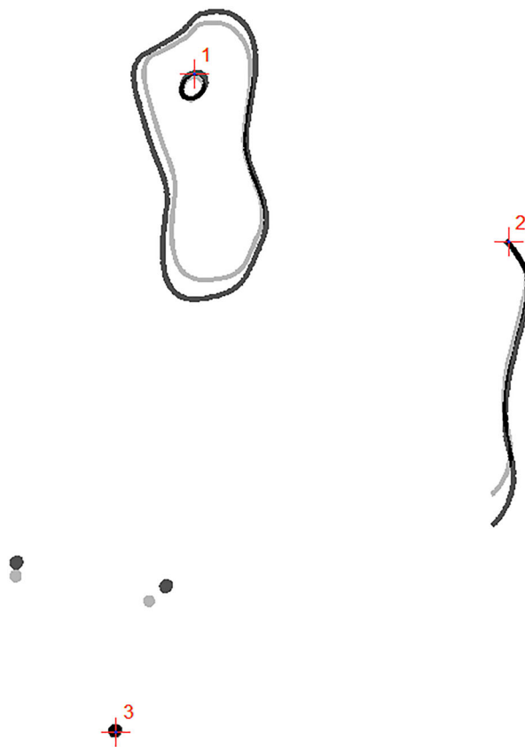
Figure 4. Illustration of the hypothetical example after transformation based on three identified control points (1,2,3) in GIS software with an affine transformation. Note in particular how the boundaries of the area fail to correspond, despite the fact that they initially had identical shapes and dimensions. Also note that only one of the three points corresponds after the transformation compared to Figure 3. The points that are numbered are those that have been used in the transformation.
