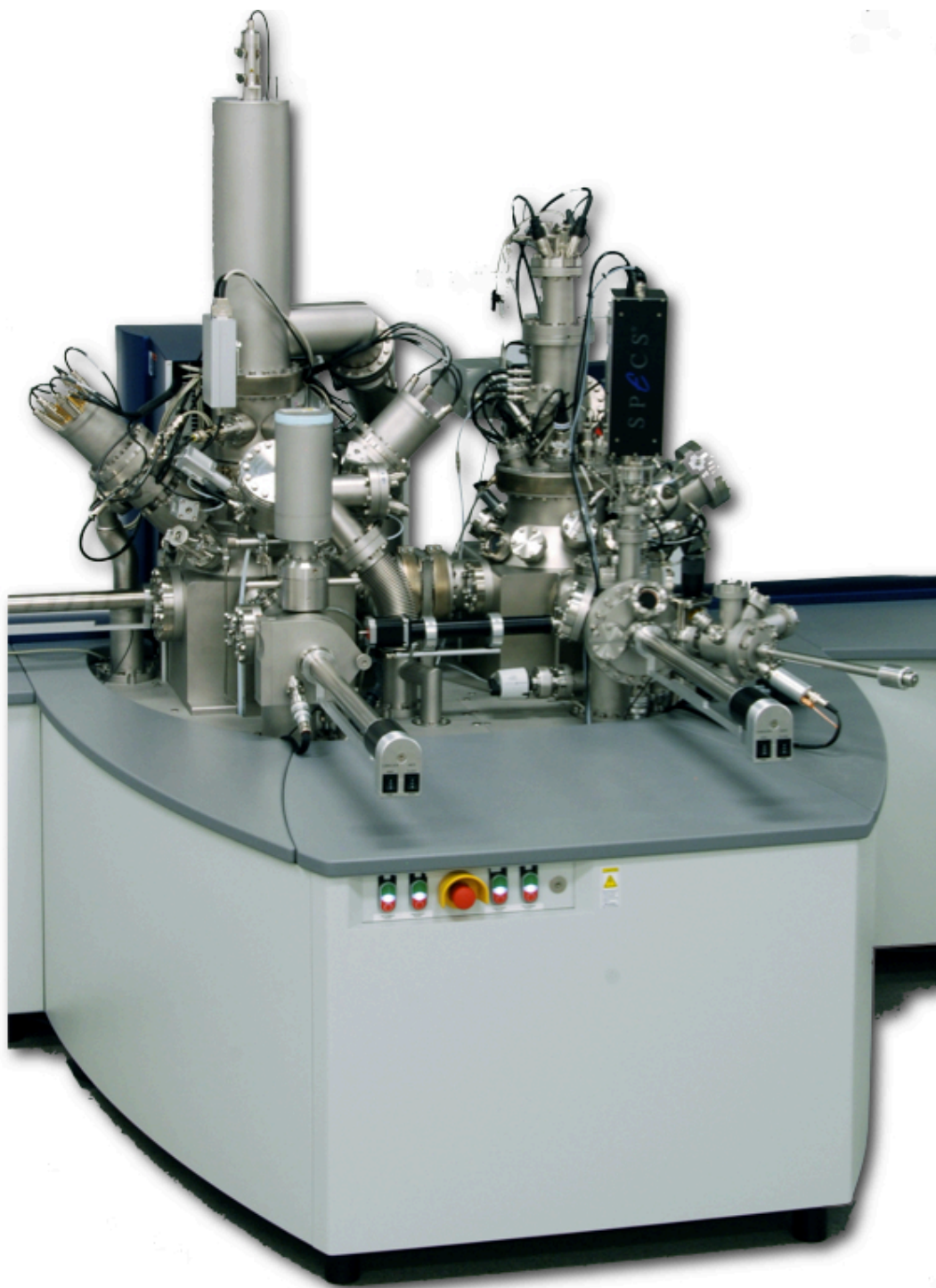
Figure A5.10. TOF.SIMS 5 and Qtac 100 instruments (left and right, respectively), with their main chambers connected. Figure used with permission from IONTOF.
