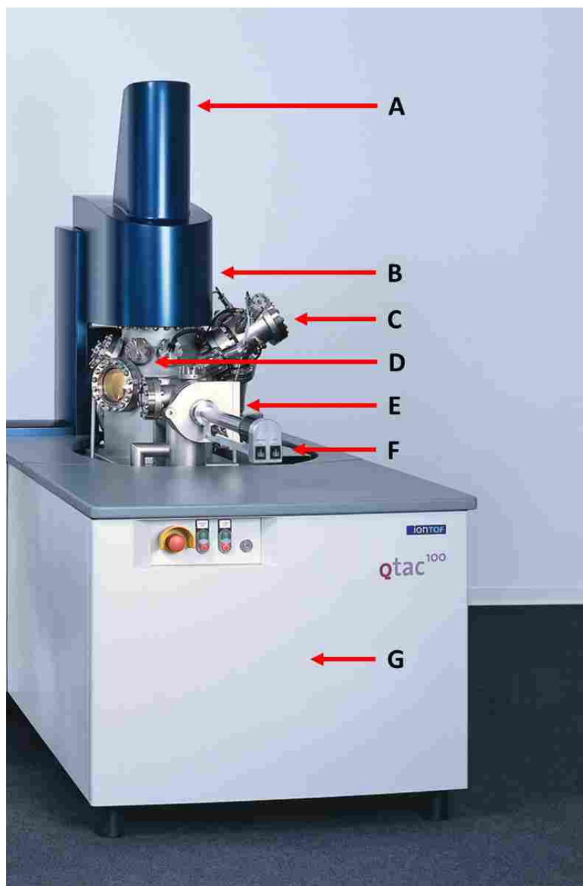
Figure A5.9. LEIS Qtac 100 instrument with locations of key components labeled. (A) Ion source. (B) Ion gun. (C) Sputter gun for depth profiling. (D) Analysis chamber (the double toroidal analyzer is located at the top of this chamber). (E) Sample introduction chamber (load lock). (F) Sample manipulator (transfer) arm. (G) Vacuum pumps and other hardware are housed below the instrument. Figure used with permission from IONTOF.
