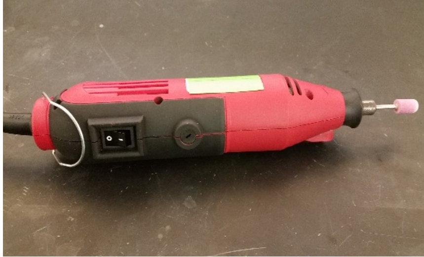
Figure A0-3 Dremmel tool used to roughen backsides of EXG™
