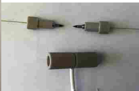
Supplemental Figure S2. Interface between the nano-flow UHPLC system and Orbitrap MS. (A) Connection between the injection valve and electro-spray source and (B) zero-dead volume union used for connecting the column and transfer line from the pump.
