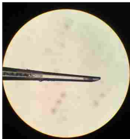
Supplemental Figure S1. Column with integrated electrospray tip. (A) Column packed with 1.7 \mu\text{m} C18 and (B) pulled electrospray tip.
