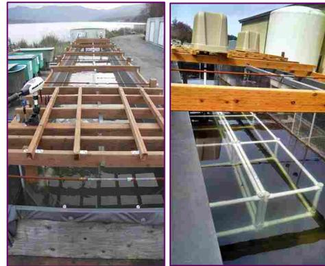
For the indoor, low-flow rate tank tests, water exchange rates were maintained at 30% volume
