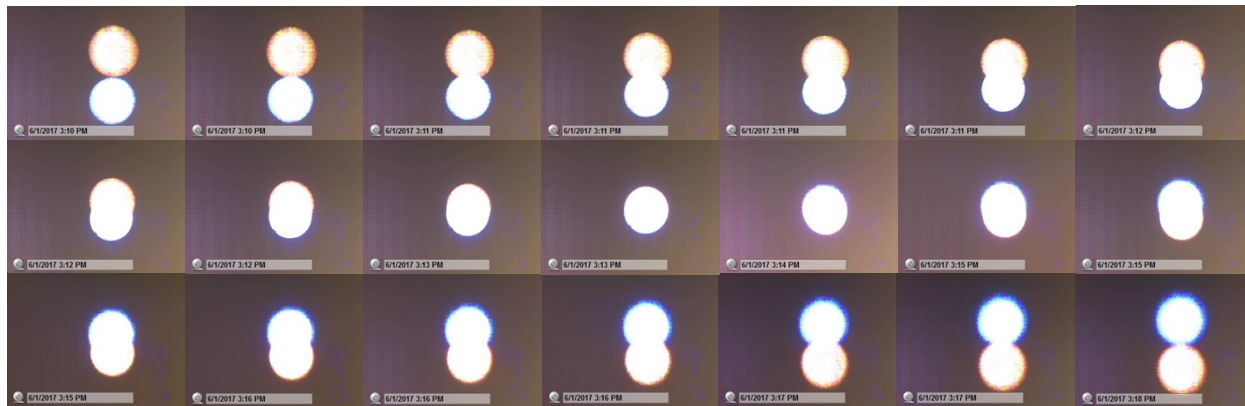
Figure 3.8 Cross over volume mapped onto a webcam. Both fibers were back lit and focused on a webcam. The distance between the optical assembly and the camera were varied incrementally until the two beams were resolved at either extreme. Images are rotated 90 degrees.
