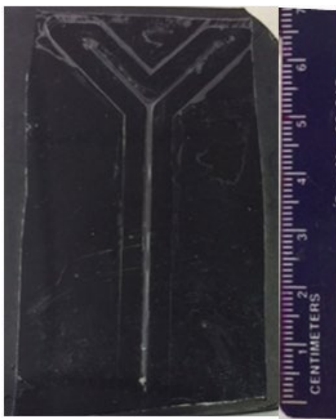
Figure 4- A typical polypropylene chip with a Y channel.
