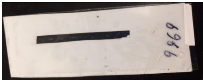
Figure 13- A channel cut out of white 9965 double-sided adhesive that was placed directly above an imprinted channel with a 9969 layer. Different films were layered on top of 9965 for auto-fluorescence experiments.
