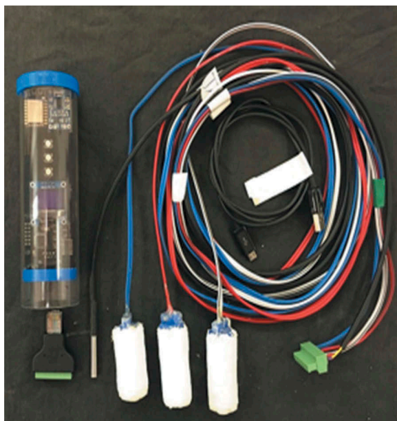
Figure 3. Chameleon soil moisture sensors and reader (Virtual Irrigation Academy, 2019).
