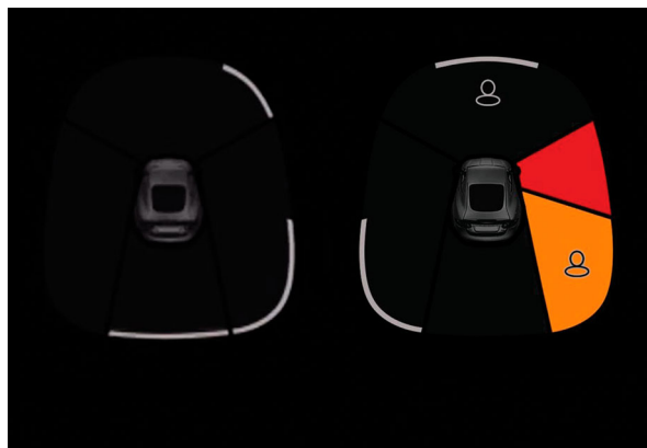
Figure 1. ATIS interface. To the left, three road users are at a distance (represented by the white lines) behind, to the back right and front right of the car. To the right, there is a pedestrian at a distance in front of the car, and another quite close in the right back blind spot. Some sort of vehicle is very close to the car's right side.
