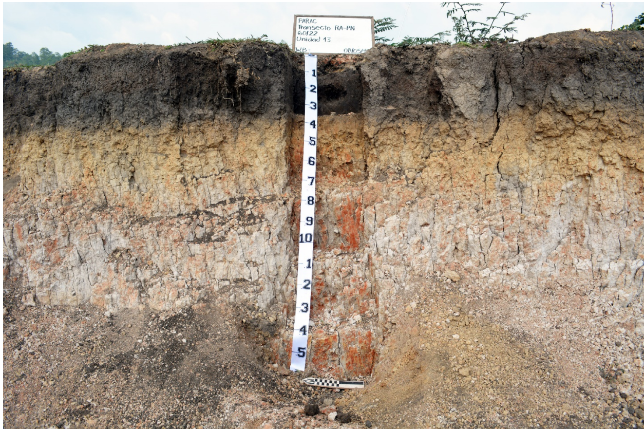
Figure 9. Profile RA13 is a toeslope profile at the base of the large hill where RA12 was taken. RA13 is from the Aquic Dystrustepts subgroup. Mottling, a redoximorphic feature, is evident below the A horizon (at 35cm) and confirms that the soil is regularly experiences very wet conditions for an extended time (during the rainy season) and dry conditions during part of each year. If a mass erosion event had occurred, there would be a layer with increased gravel and sand content deposited in this area; however, no such layer was observed.
