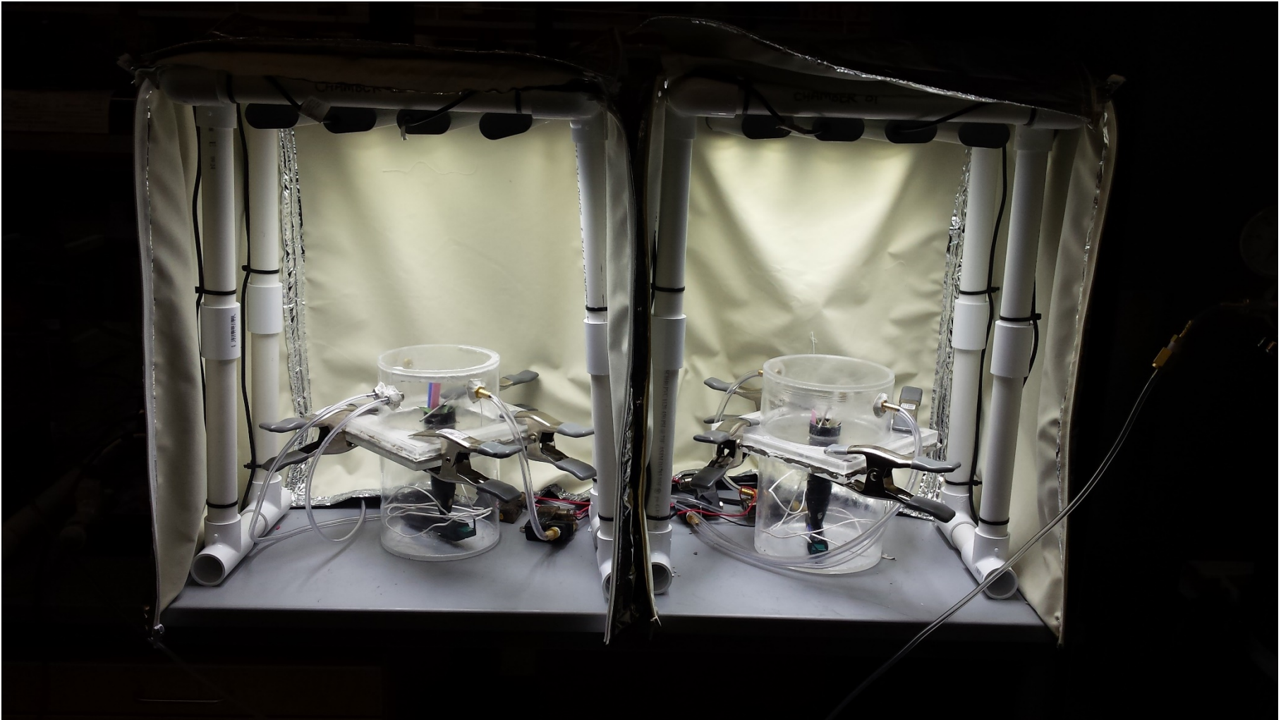
Fig. 3. Pictured are the acrylic seedling gas exchange chambers with seedlings being measured contained within.
