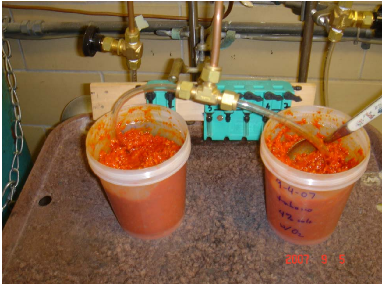
Figure 3.1.1. The apparatus for adding oxygen to mash samples before fermentation.
