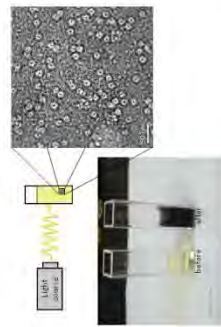
Figure 3. A light source illuminates ferritin in solution. This initiates a photocatalytic process that causes electrons to be excited and captured by an electron acceptor. The result is a metal nanoparticle with an intense color change.
