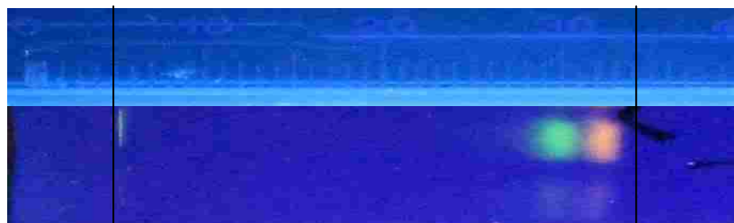
Figure 5.10 Separation of two fluorescent dyes (eosin Y disodium and sulforhodamine B) over a 30 mm run distance using a 1:100 LiCl/methanol mobile phase. The analyte concentration in the lower track is ca. 10% of the concentration of the analytes in the upper track. The fluorescent image was captured under 254 nm light.
