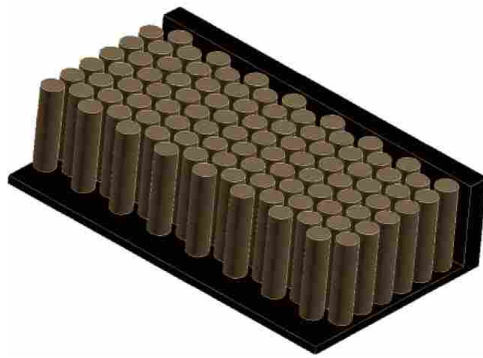
Figure 1.1 'Schematic representation of a 2-D ordered porous pillar column.' From Ref. 29 with permission.
