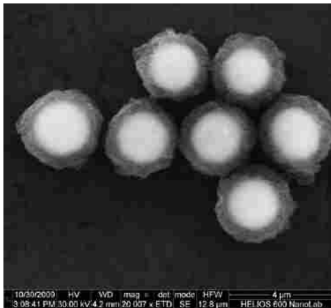
Figure 4.6 Core-shell zirconia particles imaged with different accelerating potentials: (top) imaged at 5 keV, (middle) imaged at 20 keV, and (bottom) imaged at 30 keV.
