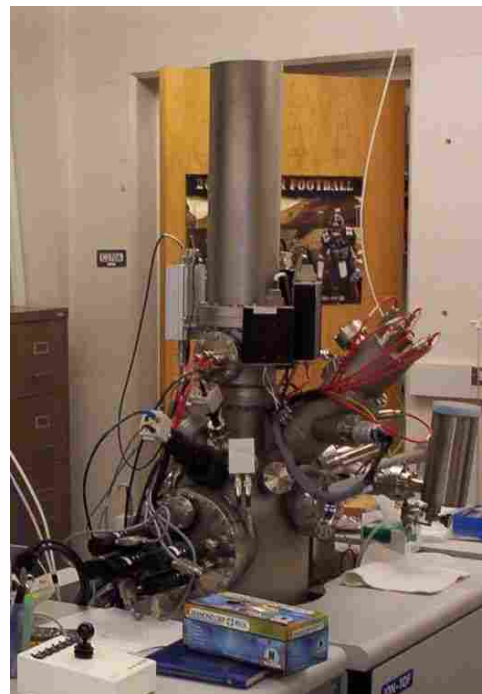
Figure 1.3. Schematic drawing of time of flight secondary ion mass spectrometry (ToF-SIMS) and a photograph of the ION-TOF IV system at BYU.
