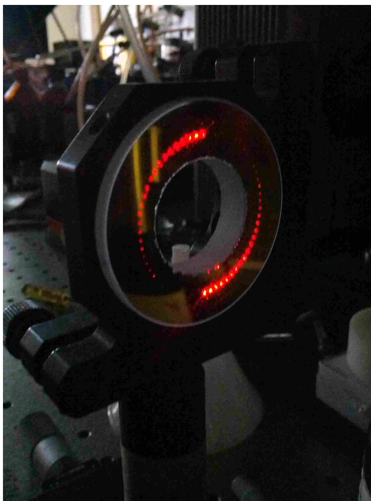
Figure 3.3: Custom Harriot cell optics facilitating excimer light pass through and 35–100 laser passes intersecting the excimer photolysis region.
