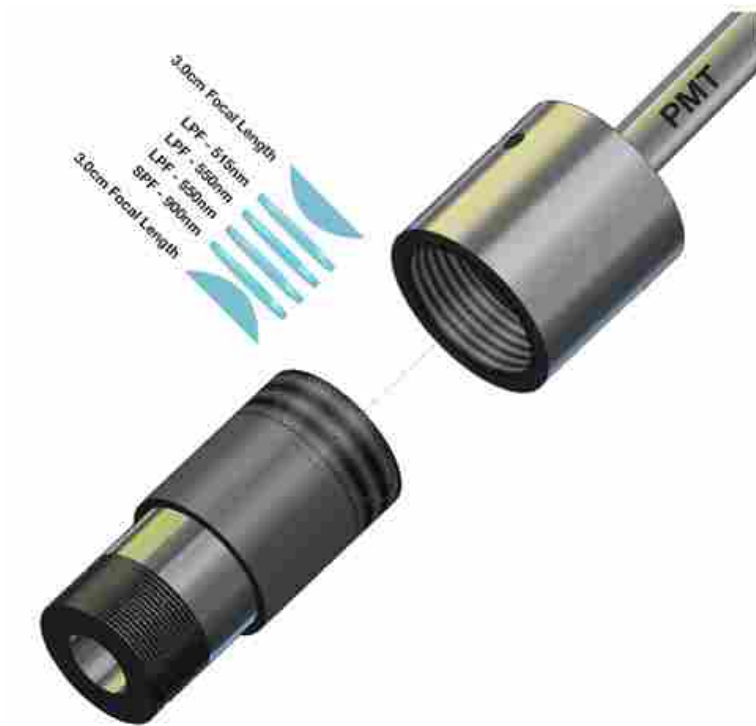
Figure 3.6: Filter tower designed to collimate fluorescence, filter noise, and then focus light onto PMT detector.
