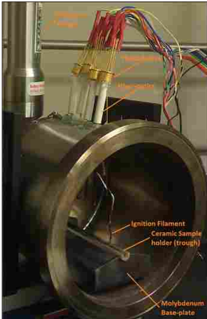
Figure 8 - 2. The Pressurized burn chamber with optical fiber/photodiode pairs for burn rate measurements and pressure gauge for gas generation measurements.
