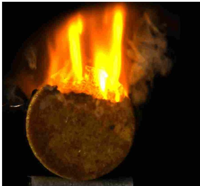
Figure 9 - 2. Image of perchlorate-ferritin pellet burning at 500 PSI. Ferritin is on the front facing portion of the pellet. (Image captured from Video 8-1)
