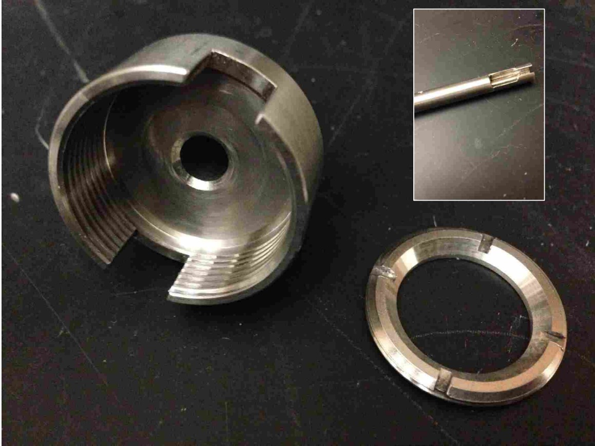
Figure 5.2 Adhesion sample holder. This holder adequately supports the sample for collecting stress data while allowing light to enter and exit the sample for the spectroscopic data collection. Inset: the post used to stress the adhesive samples can be inserted all the way through the hole in the back, and has a special channel to attach the cable that connects it with the tensile tester.
