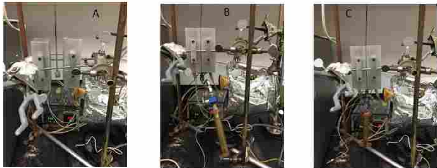
Figure 3.2 Photographs of the laboratory prototype thermal desorber. (A) pre-heated block, (B) high flow desorber with cooling tube for volatiles, (C) high flow desorber with needle trap attached for semi-volatiles.
