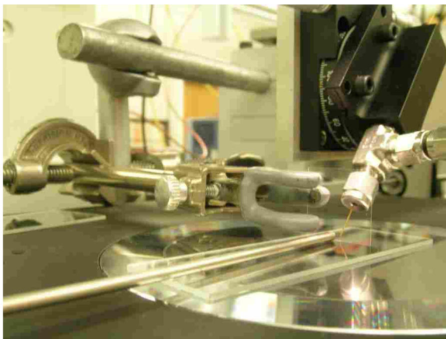
Figure 2-8 DESI barrier setup
