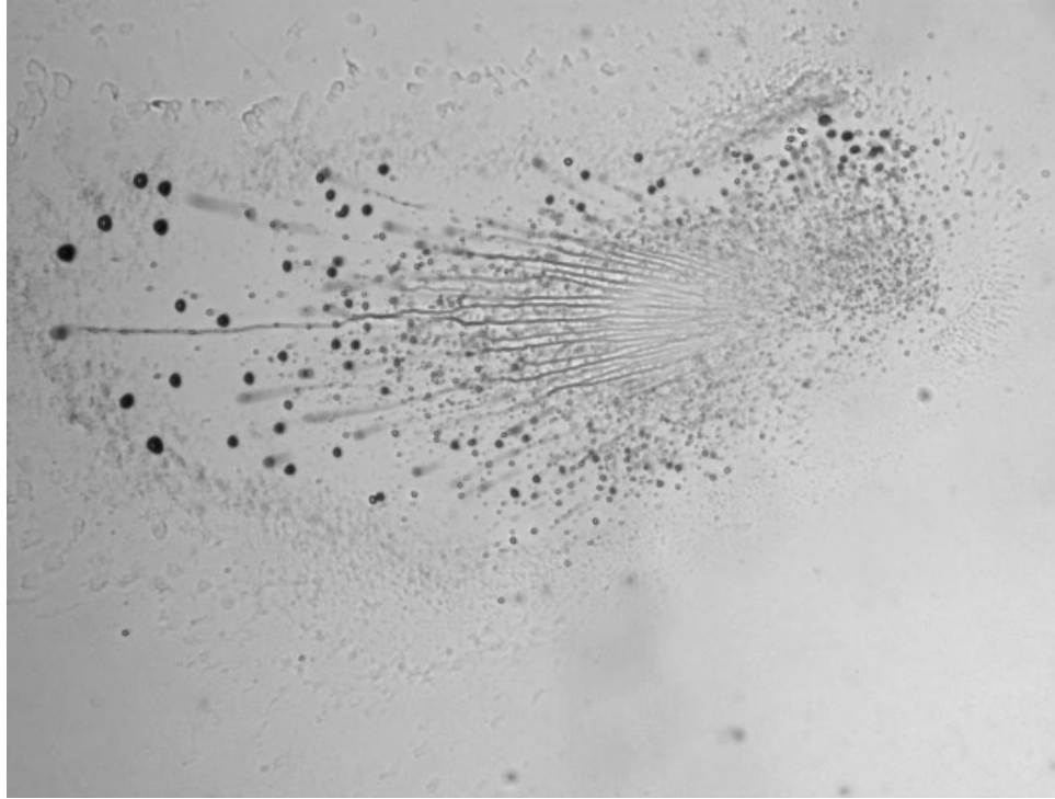
Figure 3-1 Image of the DESI spray profile of 50:50 methanol/water on glass. Taken at 3 \mu\text{L}/\text{min} 150 psi, 1.5 mm above the surface. 5 ms exposure using low level lamp light and 2x magnification. Image is 3.29 mm x 2.48 mm.
