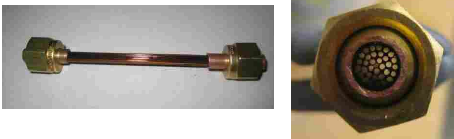
Figure 4.3. Multi-capillary trap consisting of 33 capillaries bundled together.
