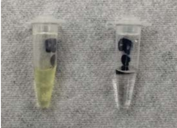
Figure 3.3. AMT treated bar origami color change. A yellow color change is observed when bar shaped origami and AMT are irradiated by UV light (left). Unmodified bar shaped origami is on the right.
