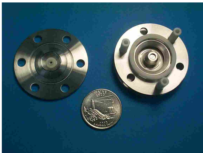
Figure 2.1. Photograph of the miniature toroidal IT mass analyzer showing the filament endcap (left) removed to expose the ion storage region (right). A U.S. quarter-dollar coin is included in order to emphasize the small size.
