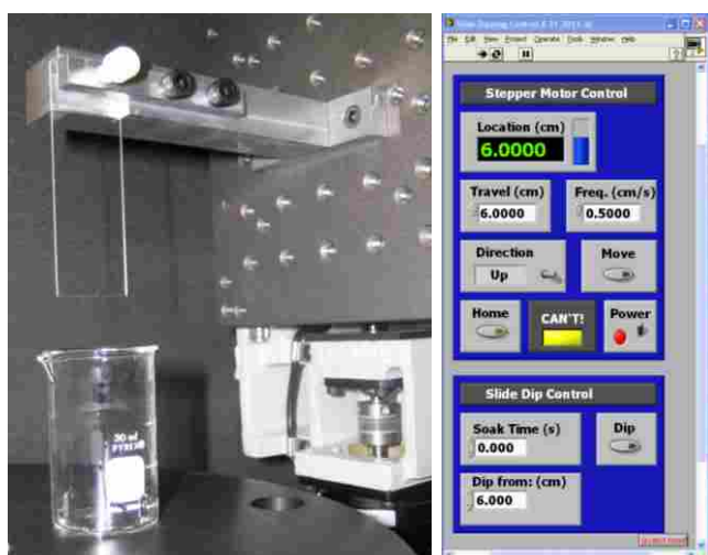
Figure 2.4: Slide dipper and controller software interface.
