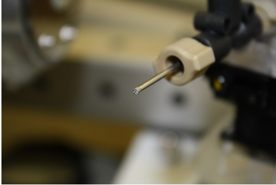
Figure 11. Picture of the electro spray needle with the nebulizing gas setup.
