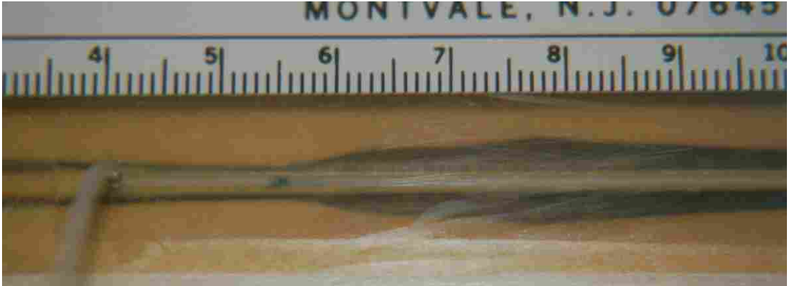
Figure III.14. Focused band of BSA in the upper channel of a two-layer channel EFGF device.
