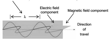
Frequency (v) of a wave is the number of cycles of the wave that pass through a point in a unit of time. Unit=waves/s or  $s^{-1}$  (hertz).
