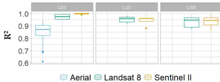
Figure 7. Box plots of enhanced aggregate no-change normalization (EANR) coefficient of determination ( R^2 ) results for each source of imagery and season across all image bands. Leaf on dormant (LDS), leaf on growing (LGS), and leaf off winter (LWS) season box plots are displayed from left to right. Aerial imagery was only acquired during LDS and is absent from LGS and LWS.
