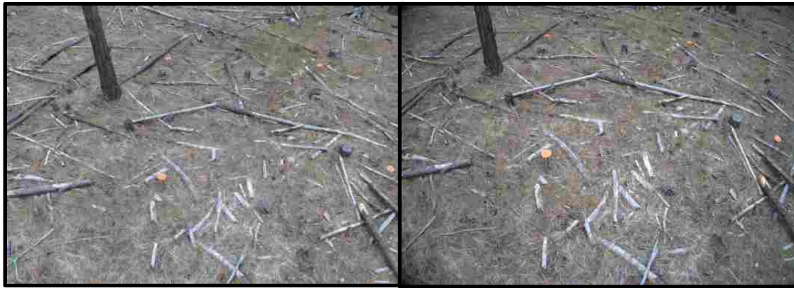
Figure 4. Left: 3-D point cloud of plot burned in May, 2017, created from structure-from-motion photogrammetry containing x, y, z spatial location and R, G, B color intensity for each point. Right: Image of same location. Spatial differences are largely due to geometric distortion, which is rectified in the point cloud.
